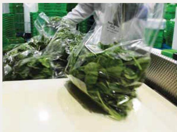
*Fresh produce is weighed, bagged and batched at impressive speeds.*
