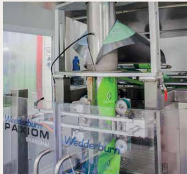
*XPdus Vertical Form Fill Sealing machine automates the process of forming, filling and sealing bags.*
