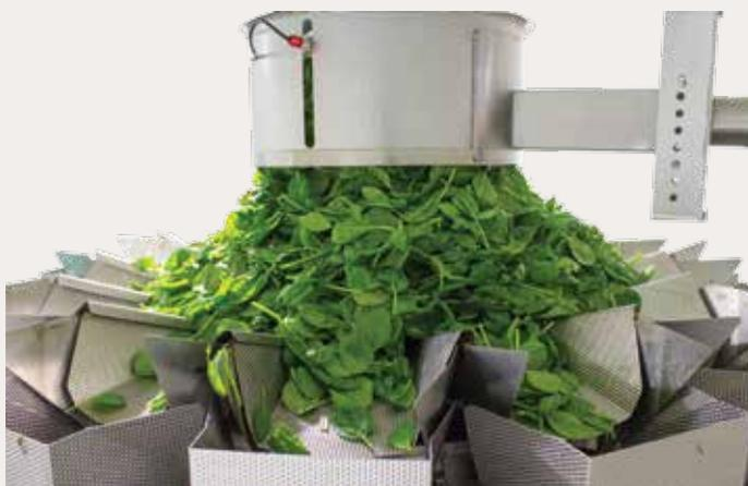
*PrimoCombi 5L Multihead Weigher with 14 head combination scale efficiently, delicately and accurately weighs fresh produce.*
